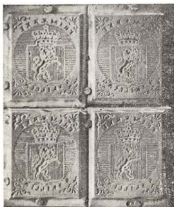
Fig. 8. Printing plate 1 for NORWEX blocks.
