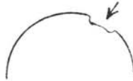
Figure 9—Perf hole cutter used by forger in Figure 1 had a nick or dull spot, as shown by little tab in perf holes across top at “7 o'clock,” and in perf holes across bottom between “11 and 12 o'clock.”
